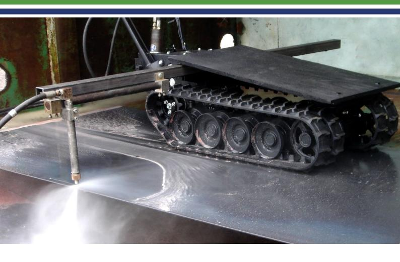
Future makes sure that the remaining cut can be weld prepared and burr free and has no impact on the associated steel allowing extremely thick and hard steels to be cut without creating a heat affect zone.
